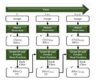
Timeline of the item identification and tracking process used by the item identification- Tracking system. class and BBox are gathered from object detection, the object tracking algorithm assigns an identification and generates predictions about the item's future location based on the current and historical BBox.
