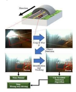
To solve these problems, researchers in [7] developed a deep learning-based Tunnel CCTV Accident Detection System. In order to train, we used the deep learning model faster R-CNN. Another model trained on image datasets that contained occurrences in tunnels served as the basis for this model. Then, ODTS uses the Car Accident Detection Algorithm (CADA) to regularly use the tracking information of the target Car object to generate Stop and WWD
