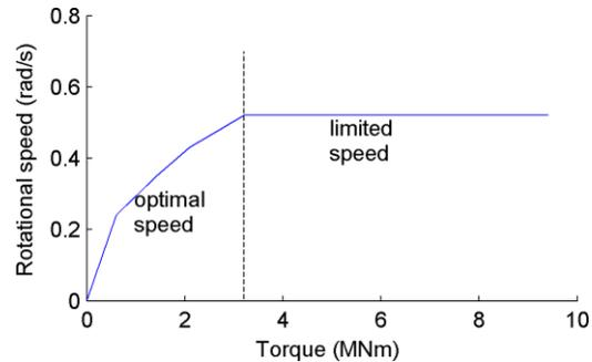
Figure 4: Torque–speed map.
