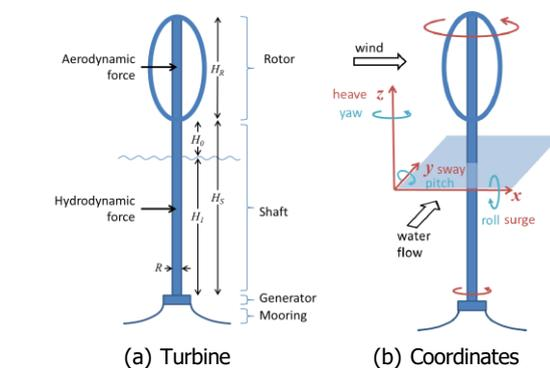
Figure 1: Schematic view of turbine and global coordinate system.
