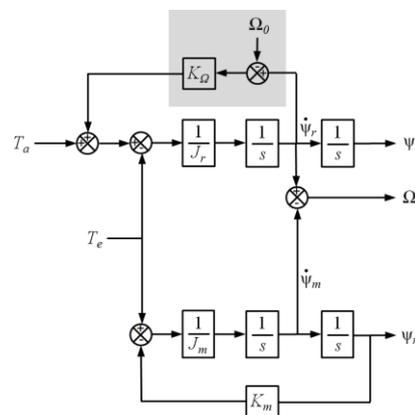
Figure 5: Simple shaft model.
