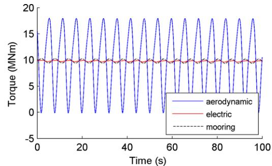
Figure 9: Variations in electric torque and torque acting on mooring system compared to input aerodynamic torque. Mean wind speed 14 m/s.
