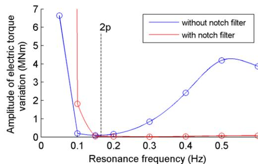
Figure 12: Amplitude of  $2p$  variations in electrical torque as a function of stator/mooring system natural frequency. Simulated results at constant 14 m/s wind.
