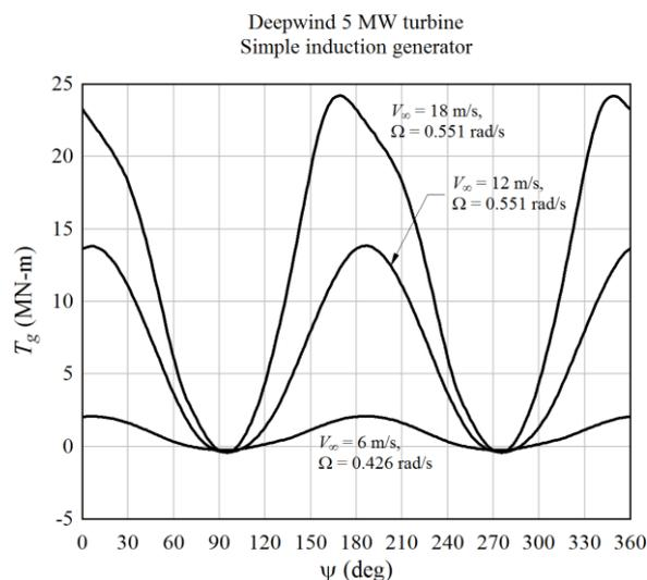
Figure 2:  $2p$  variations of the torque  $T$  with azimuth angle  $\psi$  for different wind speeds  $V_\infty$  and rotational speeds  $\Omega$ .
