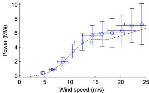
Figure 8: Simulated electrical power output versus wind speed for different stochastic wind series. Error bars indicate variability, and black dotted line represents the theoretical value.
