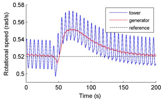
Figure 11: Rotational speed response to a deterministic wind gust that increases the wind speed from 14 m/s to about 22 m/s in the time interval 40–48 seconds.
