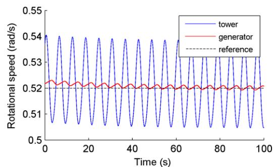
Figure 10: Rotational speed of shaft and generator rotor relative to stator. Mean wind speed 14 m/s.
