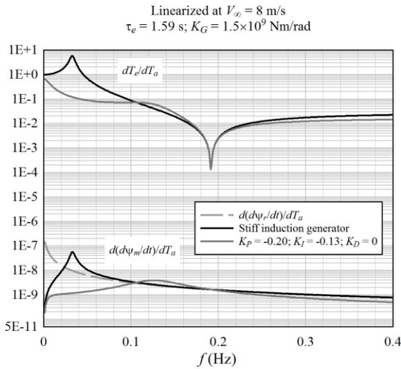
Figure 6: Frequency transfer functions for electrical and mooring system torque (top) and mooring system yaw motion (bottom) relative to aerodynamic torque.
