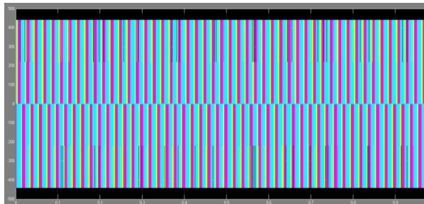
FIG 5.6 Inverter output voltage vs time before filtering
