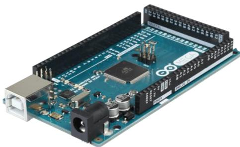
The Arduino board is a microcontroller based on the Atmega 2560 that is open-source. The processing or cabling vocabulary is handled by the board's growing environment. With their simple to use platform, these boards have reloaded the automation sector, allowing even those with little technical expertise to learn the necessary programming skills and even run the Arduino unit. These boards are used to extend interactive artifacts independently; otherwise, we'll
