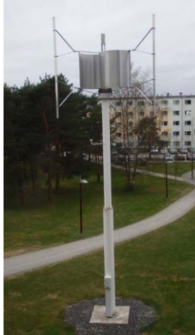
Fig. 15: It has been put in a vertical-axis wind turbine prototype generator
