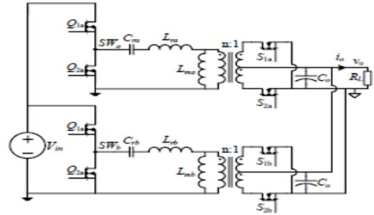
Fig. 2. Conventional two-phase LLC converter.
