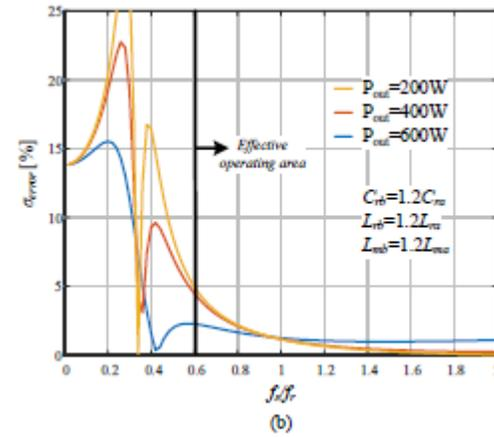
Fig. 8. Current error between the phases as a function of the switching frequency for: (a)  $C_{fb}=1.2C_{fa}$ , (b) worst case component's mismatch:  $C_{fb}=1.2C_{fa}$ ,  $L_{fb}=1.2L_{fa}$ ,  $L_{mb}=1.2L_{ma}$ .
