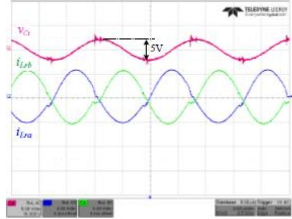
Fig. 13. Experimental waveforms of the TIFLLC converter. C2 – flying-capacitor voltage  $v_{Ct}$ (5V/div, ac coupled), C3 – phase *a* primary-side resonant tank current  $i_{Lra}$ (5A/div), C4 – phase *b* primary-side resonant tank current  $i_{Lrb}$ (5A/div). Time scale is  $2\mu\text{s}/\text{div}$ .
