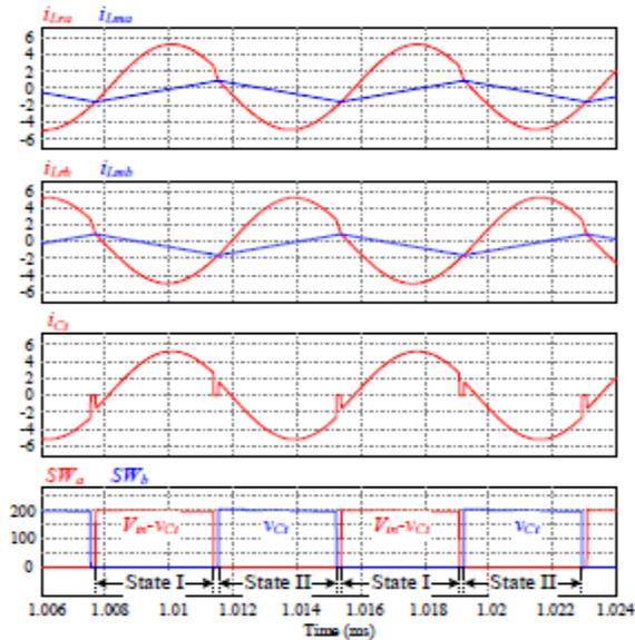
Fig. 4. Typical waveforms of the TIFLLC converter.
