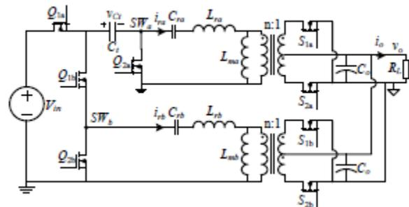
Fig. 1. *Two-phase interleaved flying-capacitor LLC (TIFLLC) converter topology.*
