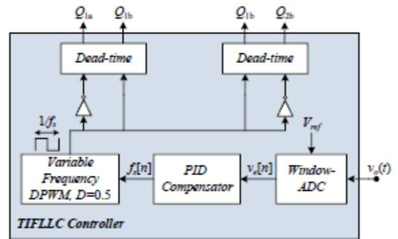
Fig. 10. Simplified block diagram of the TIFLLC controller.
