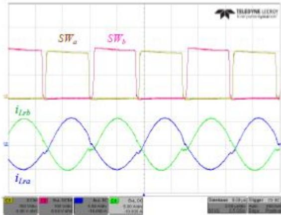
Fig. 14. Experimental waveforms of the TIFLLC converter. C1 – switching node voltage of phase  $a$   $SWa$ (100V/div), C2 – switching node voltage of phase  $b$   $SWb$ (100V/div), C3 – phase  $a$  primary-side resonant tank current  $iLra$ (5A/div), C4 – phase  $b$  primary-side resonant tank current  $iLrb$ (5A/div). Time scale is 2 $\mu$ s/div.
