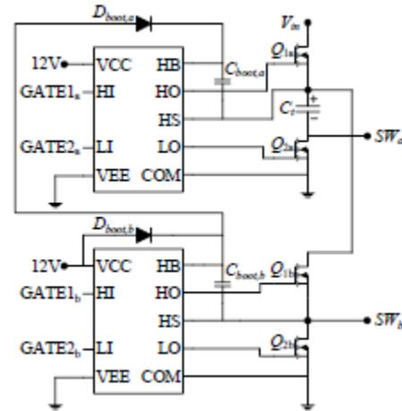
Fig. 11. Gates drivers' realization in the TIFLLC converter.
