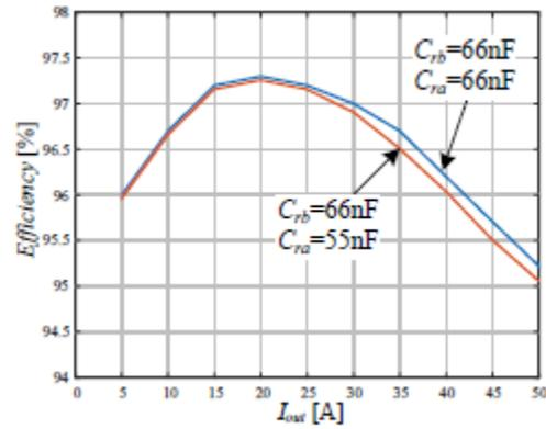
Fig. 16. Efficiency measurements of the experimental prototype.
