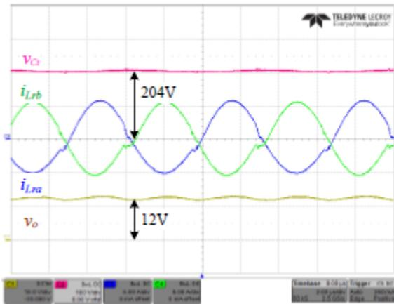
Fig. 12. Experimental waveforms of the TIFLLC converter. C1 – output voltage  $v_o$ (5V/div), C2 –
