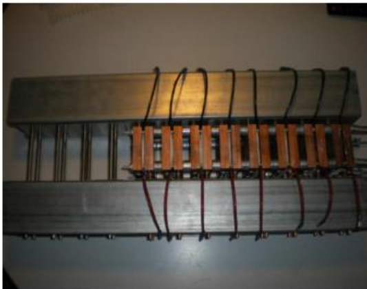
Fig. 9. An exhaust heat recovery system using heat pipes to transfer heat both to and from the TEGs.
