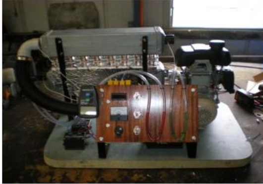
Fig. 9. An exhaust heat recovery system using heat pipes to transfer heat both to and from the TEGs.
