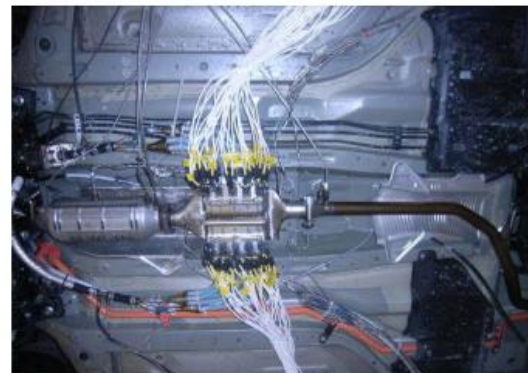
Fig. 5. Honda prototype TEG exhaust heat recovery system.
