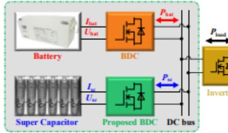
Fig. 19 Hybrid energy sources system of electric vehicles.
