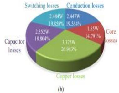
Fig. 22 Calculated power loss distributions for the experiment when  $U_{low}=40V$ ,  $U_{high}=300V$ , and  $P_n=300W$ . (a) In step-up mode. (b) In step-down mode.
