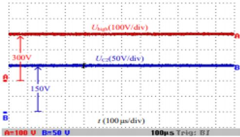
Fig. 16 Voltages across C2 and C<sub>high</sub> under U<sub>low</sub>=40V and U<sub>high</sub>=300V.
