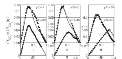
$\textbf{Fig.7.} CSE (solid lines) and CMC (dashed lines) conditional CO_2 mass fraction profiles compared to the experimental data [40] (symbols) at different axial locations.$
