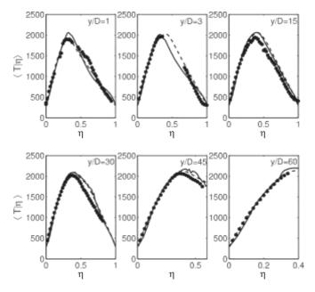
Fig. 13. CSE (solid lines) and CMC (dashed lines) conditional temperature profiles compared to the experimental data [40] (symbols) at different axial locations.
