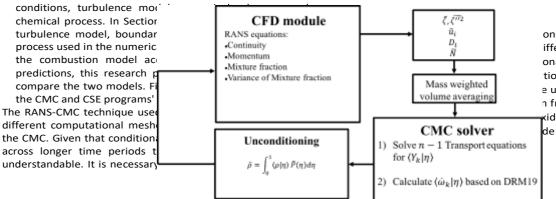
the flow and mixing field from the coarser RANS-CFD resolution to the finer CMC resolution. By averaging over a large volume of data, we can calculate the conditional velocity, turbulent diffusivity, and unconditional scalar dissipation rate [63]. Previous LES-CMC implementations have discovered that mass weighted and PDF weighted averages are both appropriate, with only minor changes in the fi-
