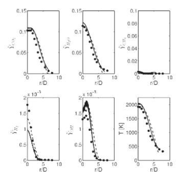
Fig.16.CSE(solidlines)andCMC(dashedlines)radialtemperatureandFavre-averagedspeciesprofilescompared to the experimental data [40](symbols) aty/D=45. Favre-averaged forecast temperatures trend in the same direction as those for the main taxa. Favre-averaged mass fractions and unconditional temperatures retrieved from the CMC and CSE.
