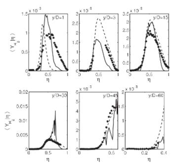
$\textbf{Fig. 10.} \ \ CSE \ (solid lines) \ and \ CMC \ (dashed lines) \ conditional \ H_2 \ mass \ fraction \ pro-files compared to the experimental data \ [40] \ (symbols) \ at different axial locations.$
