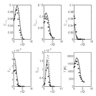
$\textbf{Fig.15.CSE} (solid lines) and \texttt{CMC} (dashed lines) radial temperature and \texttt{Favre-averaged species profiles compared} \ \ to \ the \ experimental \ data \ [40] (symbols) \ aty/D=30.$
