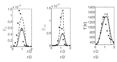
**Fig.17.**CSE(solidlines)andCMC(dashedlines)radialtemperatureandFavre-averagedspeciesprofilescompared to the experimental data [40](symbols) aty/D=7.5fortheSandiaEflame.
