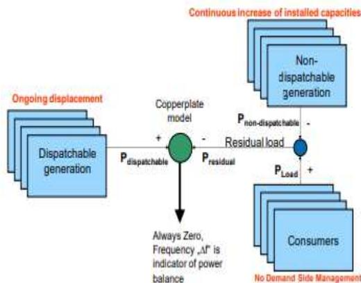
Fig. 2. A simplified scheme of the power balance of the generation system
