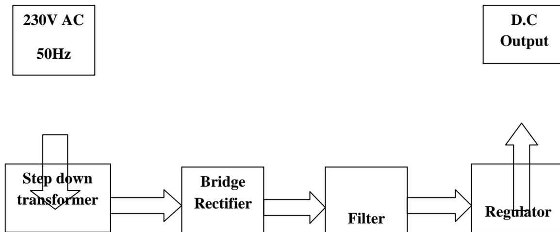
Fig: 2.1.1 Block diagram of power supply
