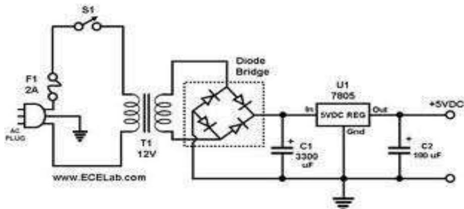
Fig Circuit Diagram of power supply
