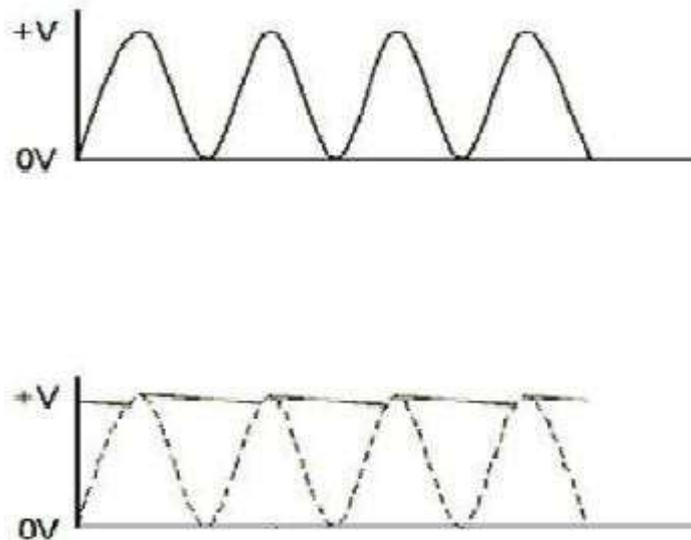
Fig 2.1.5 Waveforms of Filter Capacitor
