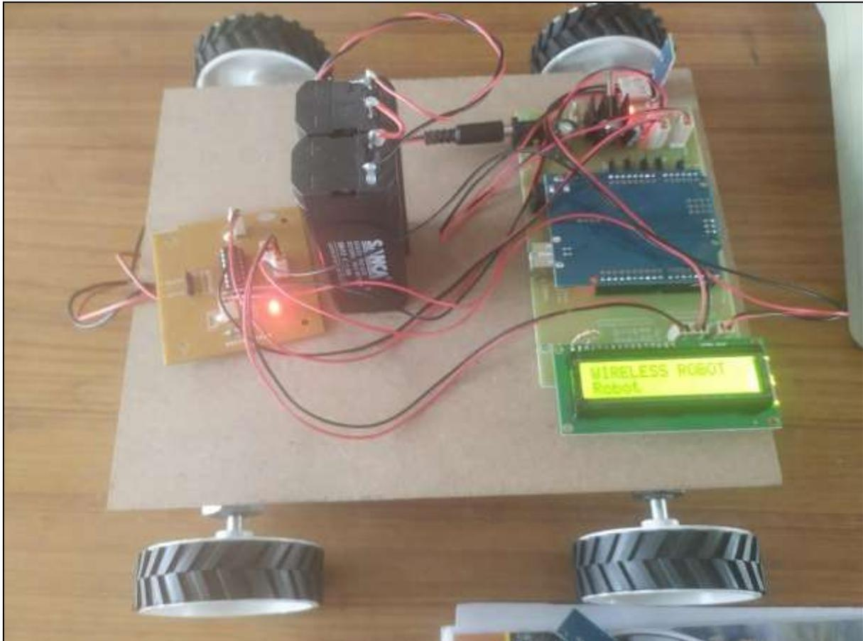
Receiver section of gesture controlled wireless ROBOT using MEMS
