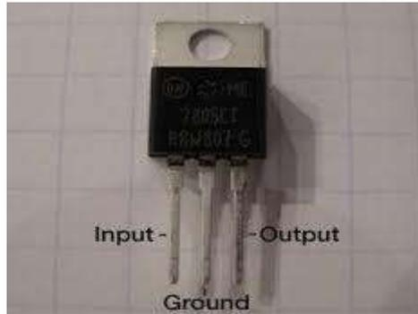
Fig 2.1.8 Pin diagram of 7805
