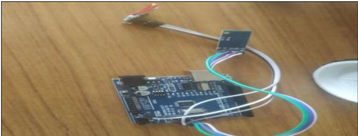
Transmitter section of gesture controlled wireless ROBOT using MEMS
