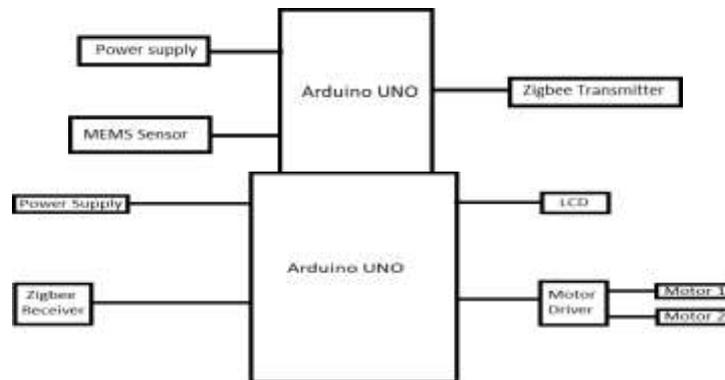
Fig: 2.1 Block Diagram of gesture controlled wireless ROBOT using MEMS.
