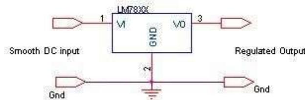
Fig.2.1.6 Pin diagram of voltage regulator
