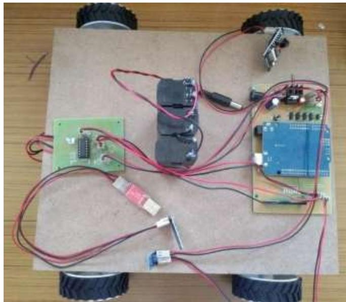
**Figure. Photocopy of Telepresence Surveillance Robot**
