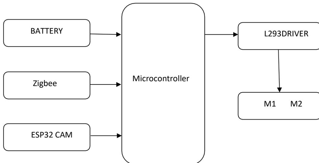
**Figure.2.1. Block Diagram of Telepresence surveillance Robot**
