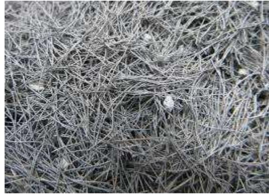
Figure no.2. Waste steel fibres
