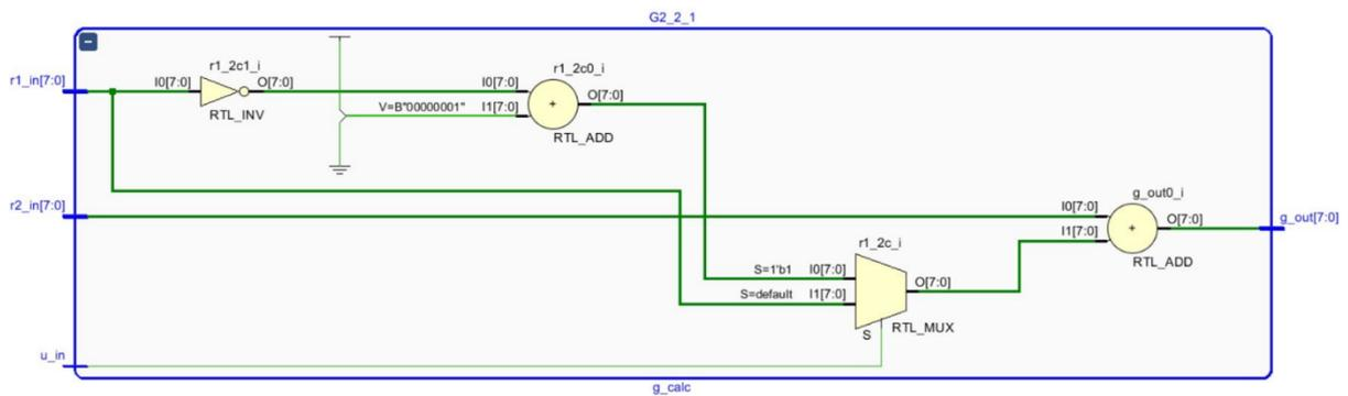
Figure.5 Schematic Decoder Polar G-cell
