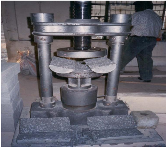
Fig 3.5.2 Split tensile strength for cylinders
