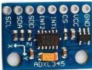
Fig3.5: ADXL345 Accelerometer
