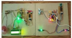
Here, the ERV and non-ERV are displayed in working state where ERV acts as a sender and non- ERV acts as a receiver. In order to replicate the speed of a vehicle, we use a DC motor. The ultrasonic sensor used in this project detects the automatic distance of the nearby vehicle and sends the information to the non-ERV which is displayed on the LCD display.
