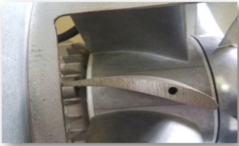
Figure 2.8. Asymmetric Aerofoil guide vanes of actual design
