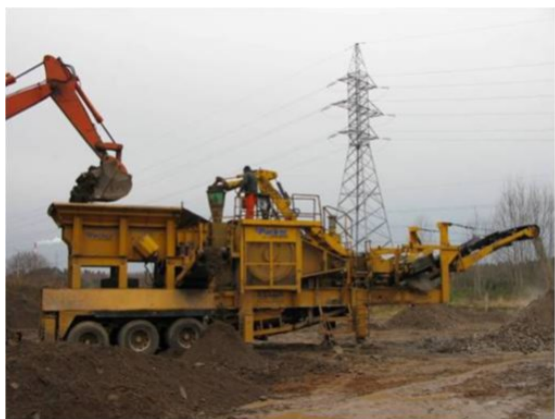
Figure2.3: Shredder used to prepare concrete breakstone on site.
