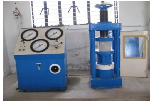
Fig 4.1 Compression strength testing
