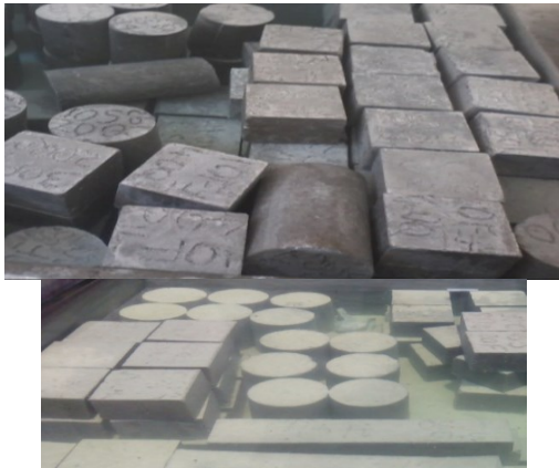
Fig 7 : Above figure shows a curing tank in which concrete specimens were kept for 3,7,28,56,90 days for hydrating of concrete.
