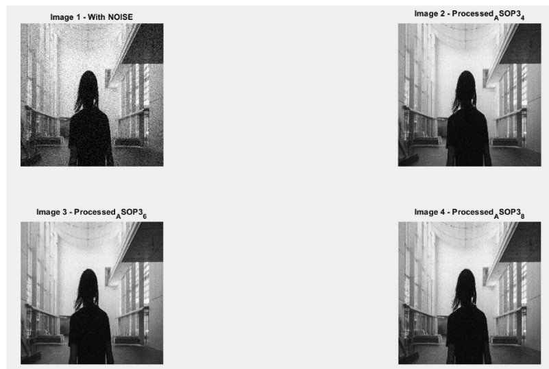
Figure.9 Image showing noise and Gaussian filter output for different ASOP3
