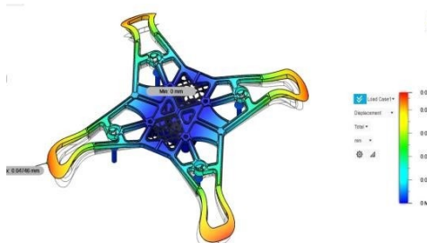
Figure 6: ABS Plastic-Total Deformation. Figure 7 : Aluminium AlSi10Mg-Total Deformation
