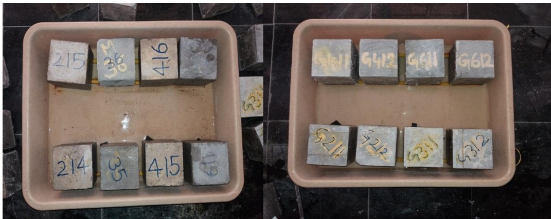
Testing of SCC and SFRSCC Specimens for Sorptivity
