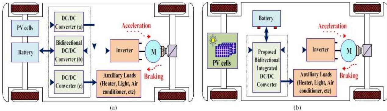
**Fig.1 Block diagram of (a) Conventional converter (b) Proposed integrated four-port converter (FPC) interface in an electric vehicle system.**
