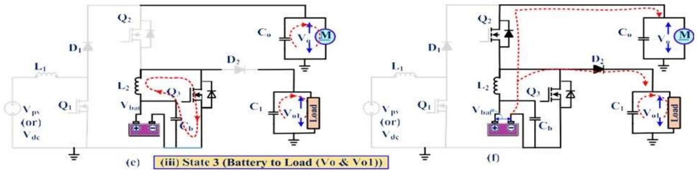
**Fig.5 State 3 (Battery to Load ( $V_0$  &  $V_{01}$ ))**
