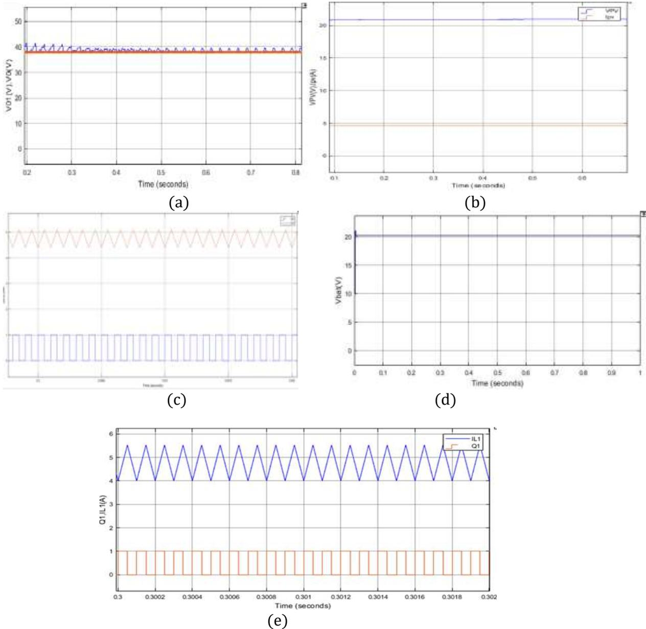
**Fig. 11: (a) Voltage ( $V_{01}$ ), ( $V_0$ ); (b) Voltage ( $V_{pv}$ ), Current ( $I_{pv}$ ); (c) Inductor current ( $I_{i2}$ ); (d) Battery Voltage ( $V_{Bat}$ ); (e) Inductor Current ( $I_{i1}$ )**
