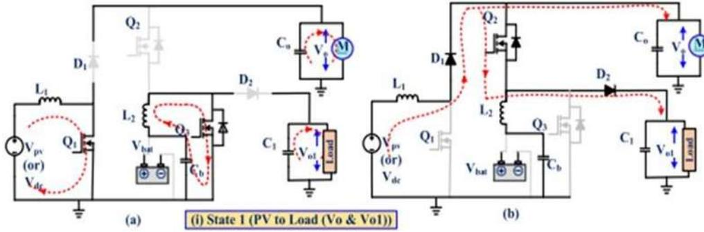
**Fig.5 State1 (PV to Load ( $V_0$  &  $V_{01}$ ))**
