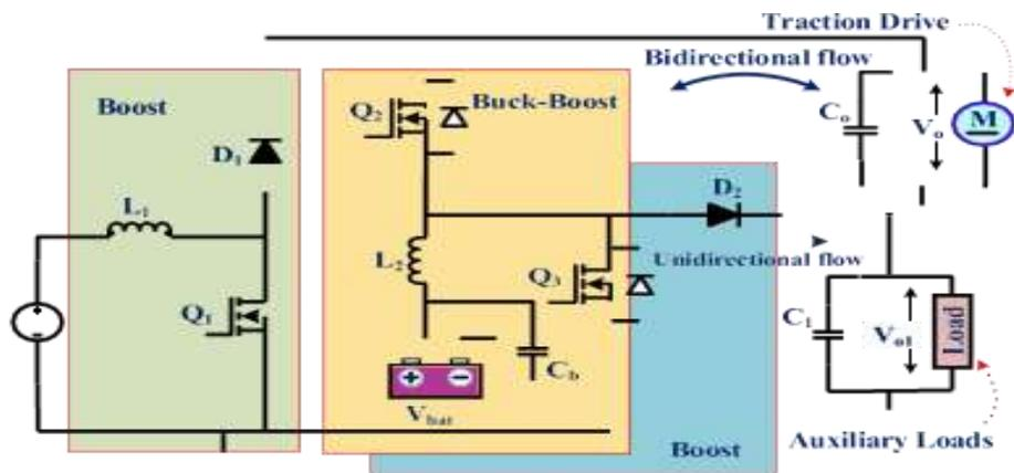
**Fig.2 Topology diagram of four-port (FPC) converter**
