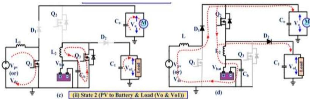
**Fig.5 State 2 (PV to Battery & Load ( $V_0$  &  $V_{01}$ ))**
