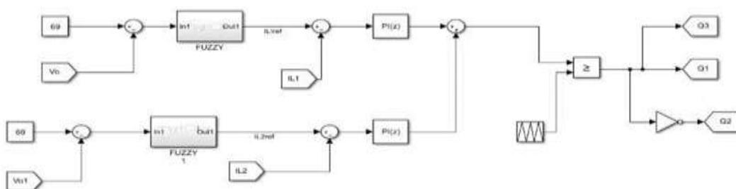
**Fig. 7 Controlling Block of FUZZY Logic Controller**
