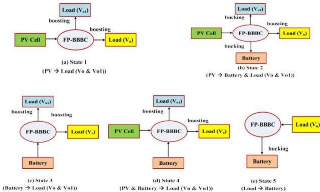
Fig.3 a) State 1(boost), b) State 2 (buck & boost), c) State 3 (boost), d) State 4 (boost), e) State 5 (buck)
