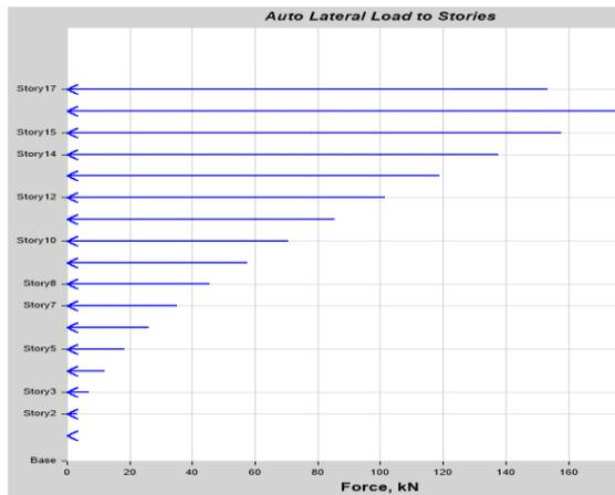
**Fig: Lateral seismic load distribution in X-direction on structure in zone III**
