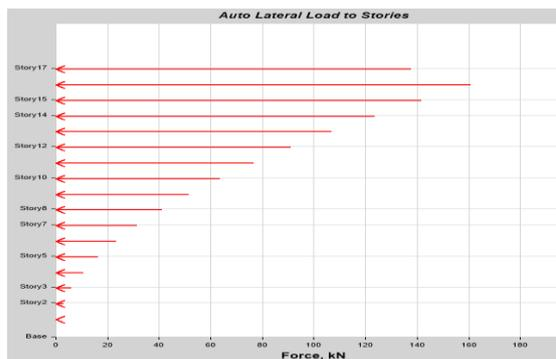
**Fig: Lateral seismic load distribution in Y-direction on structure in zone III**
