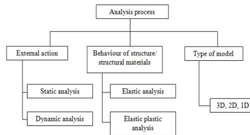
Fig : Method of Analysis Process (Syrmakezis, 1996)
