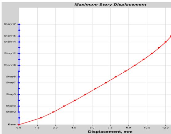
**Fig: Maximum storey displacements of structure for EQ Y in zone III**
