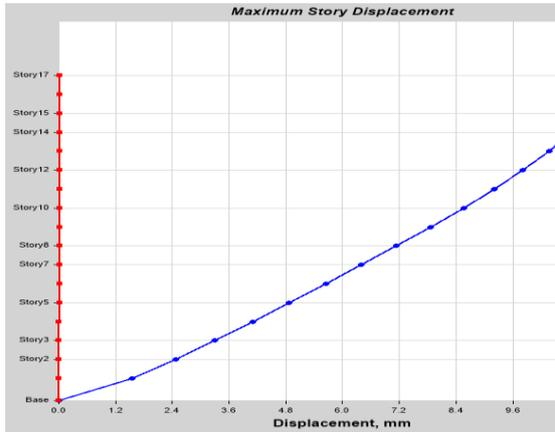
**Fig: Maximum storey displacements of structure for EQ X in zone III**
