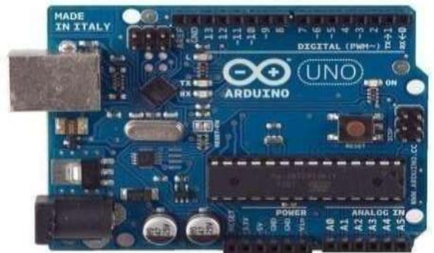
Figure 5: Arduino UNO Carrier Synchronization:
